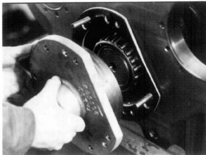
FIG. 6.1-13 Press smaller bearing cup into end cap. Using approximately .150 inches pile of shims, assemble end cap to front of housing. Extended length bolts with the heads removed can be used as simple guides to support and locate all gaskets, shims and end caps as required.
