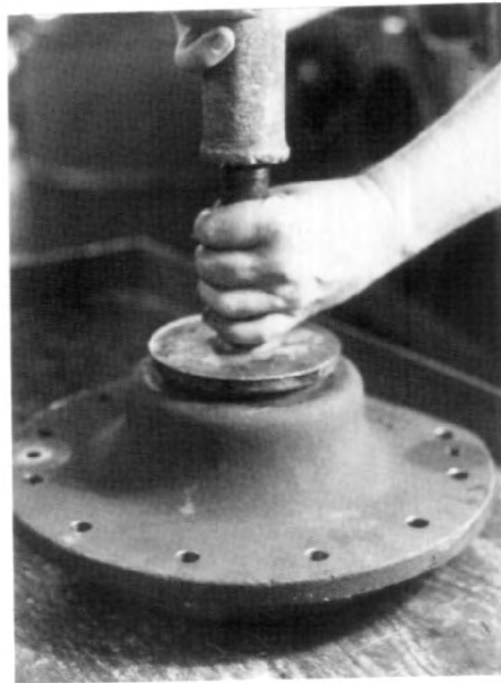
FIG. 6.4-14 Seat oil seal in speedo carrier.
