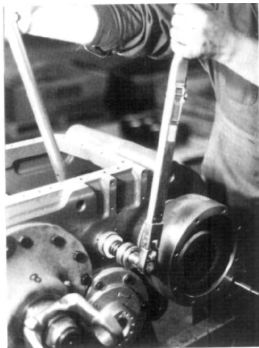
FIG. 6.6-3 Temporarily tighten hexagon locknut on shaft and while restraining locked nut, tighten locknut retaining piston to appropriate torque. Loosen shift fork locking nut.
