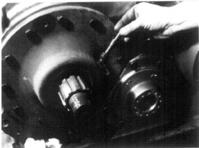
FIG. 6.4-17 Smear speedo pinion gear teeth with grease and place into carrier. Be sure teeth engage drive gear properly.
